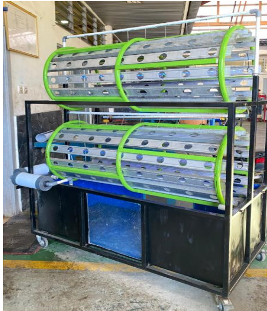
Fig 2. Prototype of a double-rotary-table-based aquaponics system following fabrication
